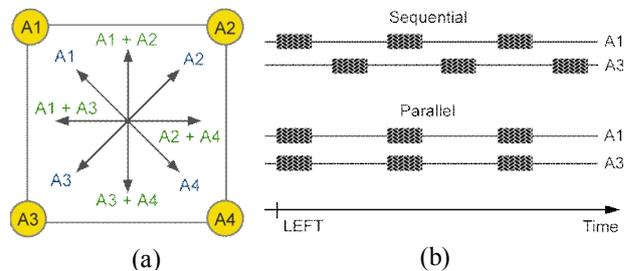
Figure 2. Stimulation model (a) and a signal timing for the encoded direction “left” in sequential mode (b).
