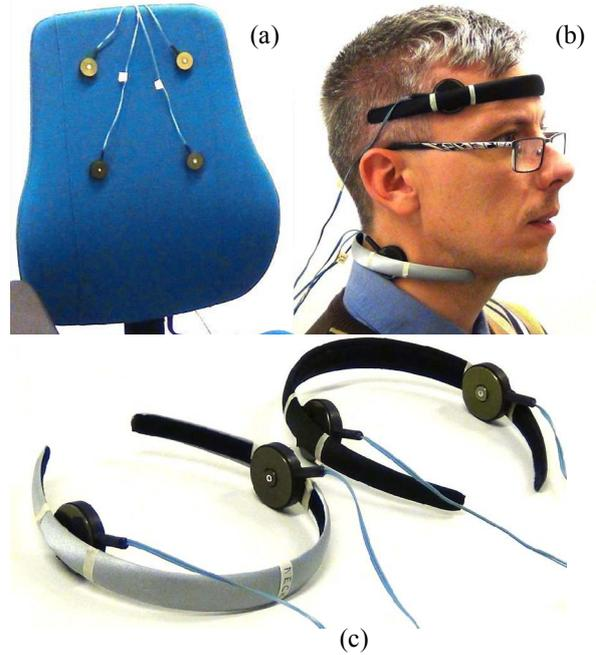
Figure 1. Experimental setup, hardware: chair-back (a) and head-neck (b) locations, hair-bands with actuators attached (c)
