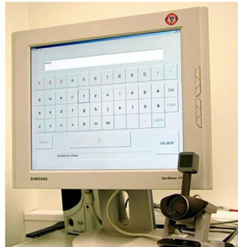
Figure 1. On-screen keyboard and eye-tracking device.
