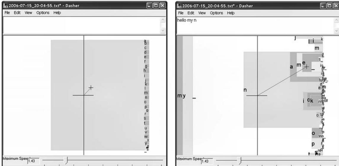
Figure 9-4. Dasher<sup>3</sup> facilitates text entry by navigation through a zooming world of letters. In the initial state, the letters are ordered alphabetically on the right side of the screen (image on the left). As the user looks at the desired letter, its area starts to grow and simultaneously the language prediction system gives more space to the next most probable letters. In the image on the right, the user is in the middle of writing “name”, with “n” already selected.
