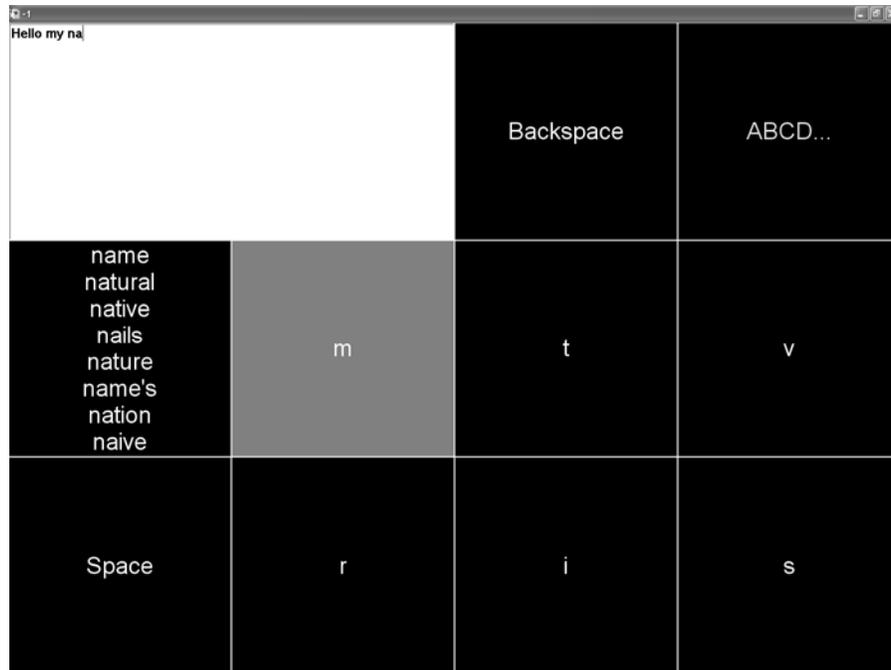
Figure 9-2. The 3x4 on-screen grid of the GazeTalk system.
