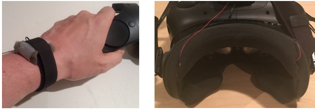
Figure 1: One actuator was on the wrist (left). Two actuators were on the participant's temples (right).
