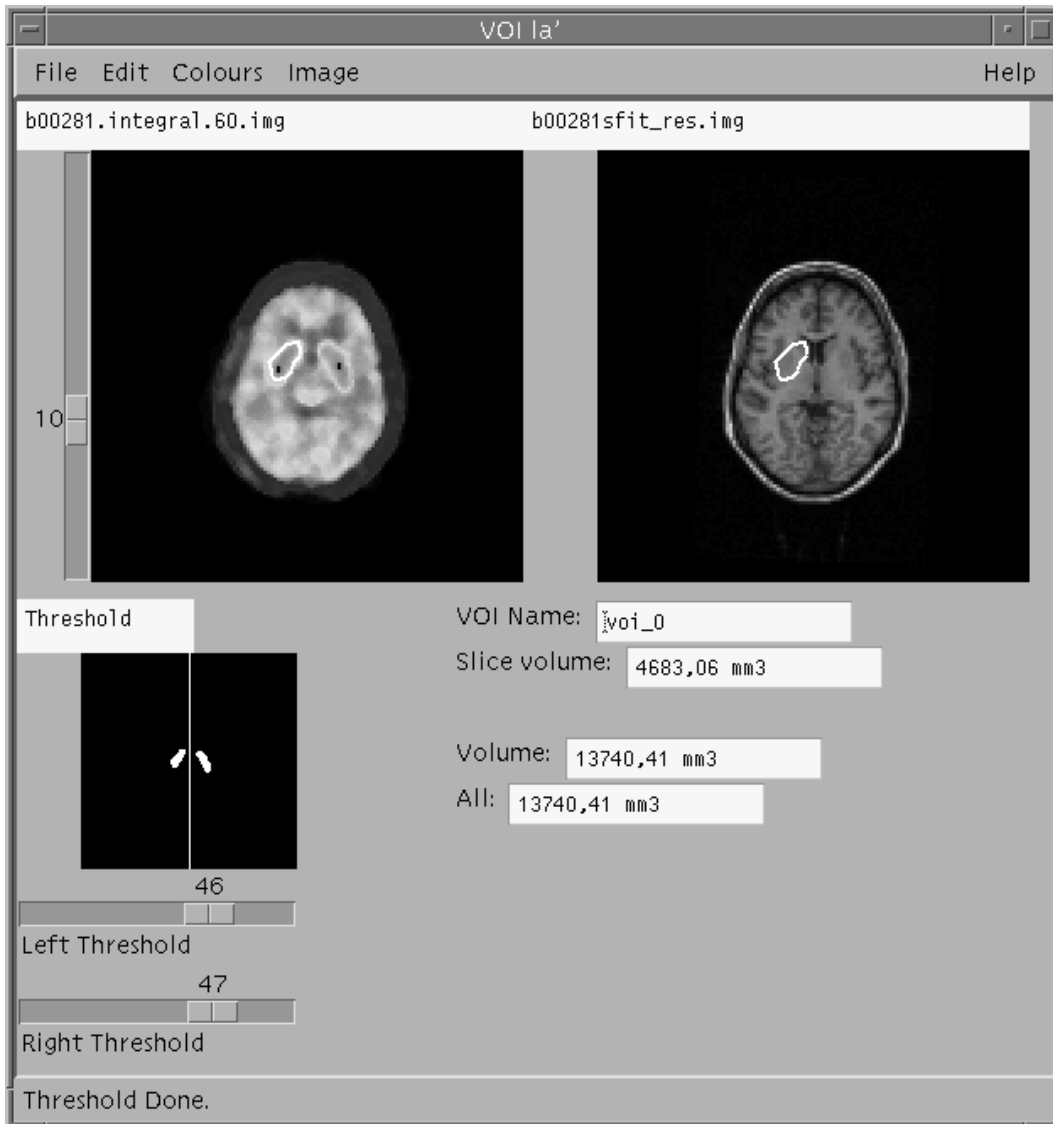
Figure 2: User interface. The upper left image is a user selected slice from a 3D image. A vertical scale on the left hand side is used for slice selection. The scale also shows the number of the current plane. The lower image shows the corresponding thresholded version of the current slice. User may select some other slice to view by dragging the scale. The horizontal scales at bottom are used to adjust threshold levels. The upper right image is optional and is used for verifying results by displaying corresponding ROIs on it. On the lower right part, the current VOI information is shown with a user editable name.
